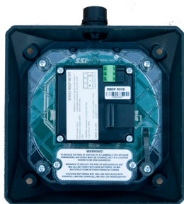
900CDP Battery and Wiring Access
